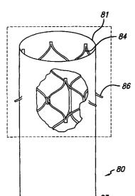
(57) Abstract: The present invention embodies an endovascular graft having an attachment frame connection mechanism that allows placement of the main body component in vasculature in combination with limb components. Various limb component - to - main body component attachment mechanisms are provided which ensure a reliable bond while facilitating a smaller delivery profile.
