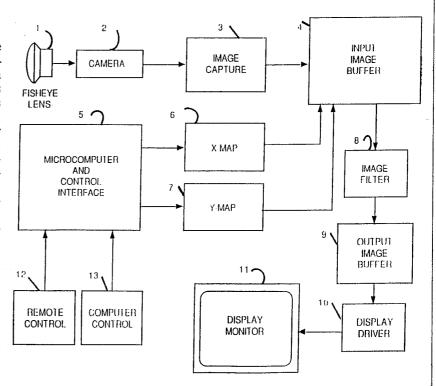
compatible with standard video equipment. The device can be used for any application where a conventional pan-and-tilt or orientation mechanism might be considered including inspection, monitoring, surveillance, and target acquisition.
