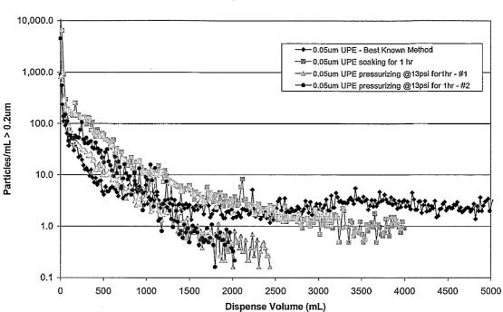
Particle Performance of 0.05um UPE filter on Intelligen 2 pump Dispense rate = 0.833mL/s, Dispense volume=5mL, Filtration rate = 5mL/s
