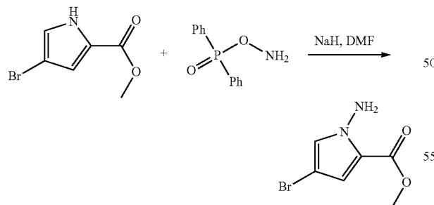
To a solution of 4-bromo-1H-pyrrole-2-carboxylic acid methyl ester (3.5 g, 17.2 mmol, 1 eq) in DMF (120 mL) was added NaH (0.82 g, 20.6 mmol, 1.2 eq) at 0°C., and the mixture was stirred at 0°C. for 1 h, followed by the addition of O-(diphenylphosphoryl)-hydroxylamine (6 g, 25.8 mmol). The reaction mixture was stirred for another 1 h, then neutralized with 20% NH<sub>4</sub>Cl solution, and extracted with EA. The combined organic layers were washed with water
