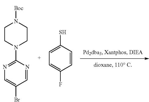
Step 1: Synthesis of tert-butyl 4-(5-(4-fluorophenylthio)pyrimidin-2-yl)piperazine-1-carboxylate
