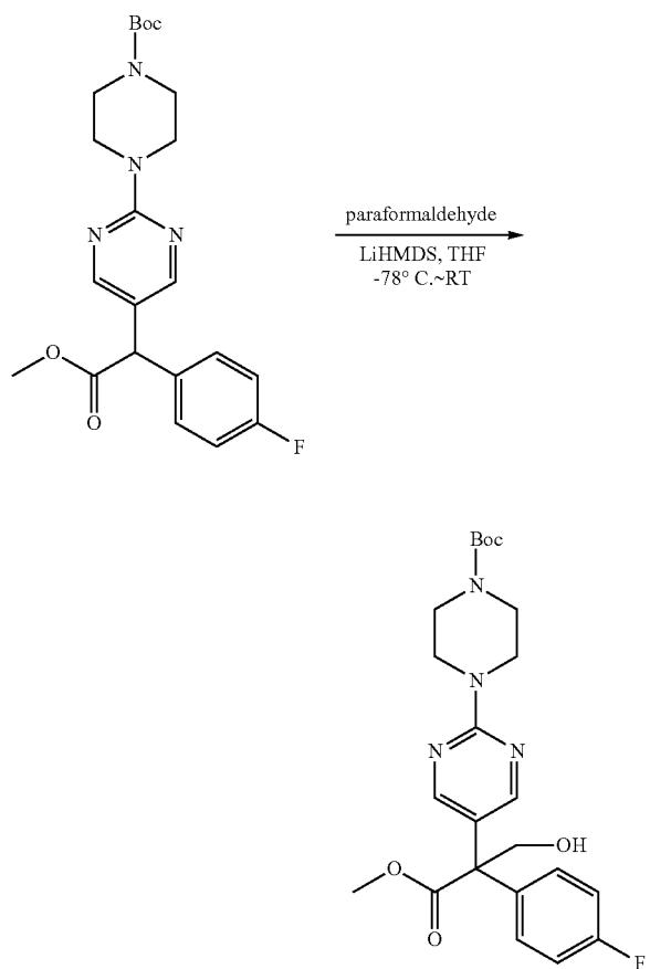
A solution of tert-butyl 4-(5-(1-(4-fluorophenyl)-2-methoxy-2-oxoethyl)pyrimidin-2-yl)piperazine-1-carboxylate (650 mg, 1.5 mmol) in THE (20 mL, dry) was cooled to -78°C and protected with N<sub>2</sub>. Another solution of n-BuLi
