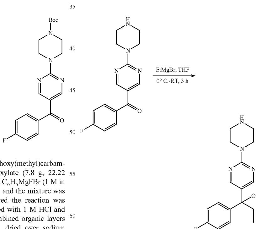
To a solution of (4-fluorophenyl)(2-(piperazin-1-yl)pyridin-5-yl)methanone (4.0 g, 21.84 mmol) in dry THF (150 mL) was added EtMgBr (1 M in THF, 150 mL) at 0°C under nitrogen. The mixture was stirred at RT for 3 h, then
