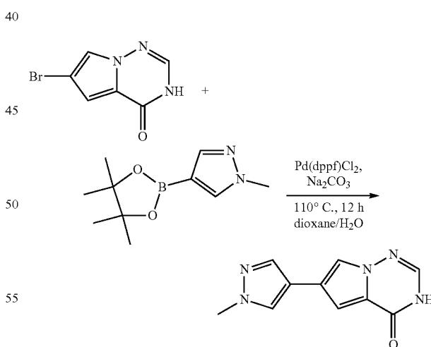
A mixture of 6-bromo-3H-pyrrolo[2,1-f][1,2,4]triazin-4-one (2.15 g, 10 mmol), 1-methyl-4-(4,4,5,5-tetramethyl-1,3,2-dioxaborolan-2-yl)-1H-pyrazole (4.2 g, 20 mmol), Cs<sub>2</sub>CO<sub>3</sub> (9.8 g, 30 mmol), PdCl<sub>2</sub>dppf (814 mg, 1 mmol), water (15 mL), ethanol (15 mL) and dioxane (70 mL) in a 250 mL flask was degassed with N<sub>2</sub> for 10 min, and then heated at 120°C. under N<sub>2</sub> atmosphere overnight. The mixture was cooled to RT, followed by the addition of silica
