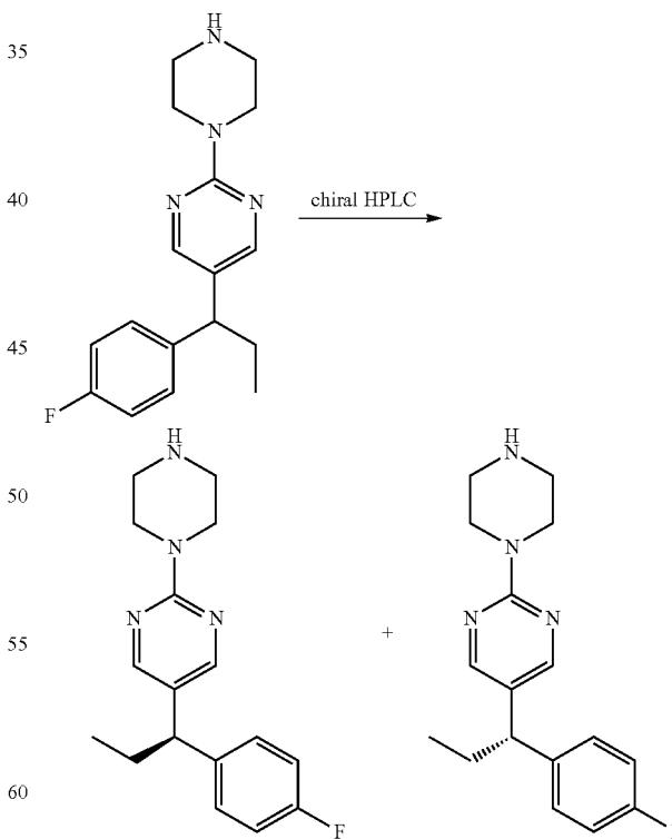
The above racemate compound (90 mg) was separated by Chiral-HPLC to afford the enantiomers (35 mg). MS (ES+)  $\text{C}_{17}\text{H}_{21}\text{FN}_4$  requires: 300, found: 301  $[\text{M}+\text{H}]^+$ . The absolute stereochemistry was assigned randomly.
