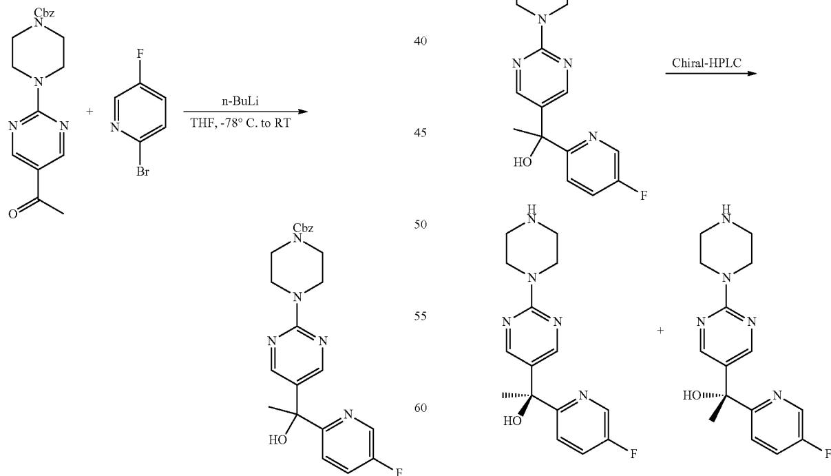
To a solution of 2-bromo-5-fluoropyridine (1.3 g, 7.50 mmol) in anhydrous THF (30 mL) was added n-BuLi (2.76
