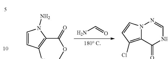
A mixture of methyl 1-amino-3-chloro-1H-pyrrole-2-carboxylate (4.00 g, 23 mmol) and formamide (15 mL) was heated to 180° C. for 3 h. After cooled to RT, the precipitated solid was collected via filtration and washed with  $\text{CH}_2\text{CH}_2$  to obtain the title compound (2.50 g, 64%) as a yellow solid. MS (ES+)  $\text{C}_6\text{H}_4\text{ClN}_3\text{O}$  requires: 169, found: 170 [M+H]<sup>+</sup>.
