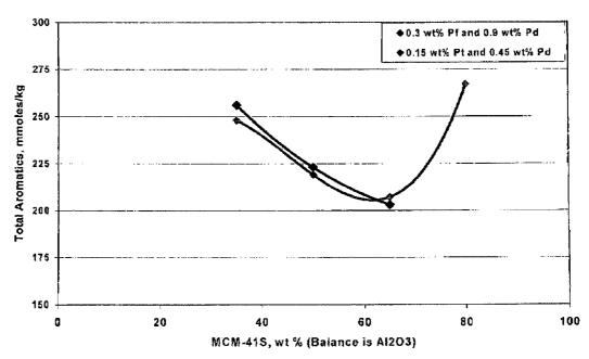
Feed: 210 ppm Sulfur, 415 mmoles/kg Aromatics, 275 C, 2 LHSV, and 1000 psig
