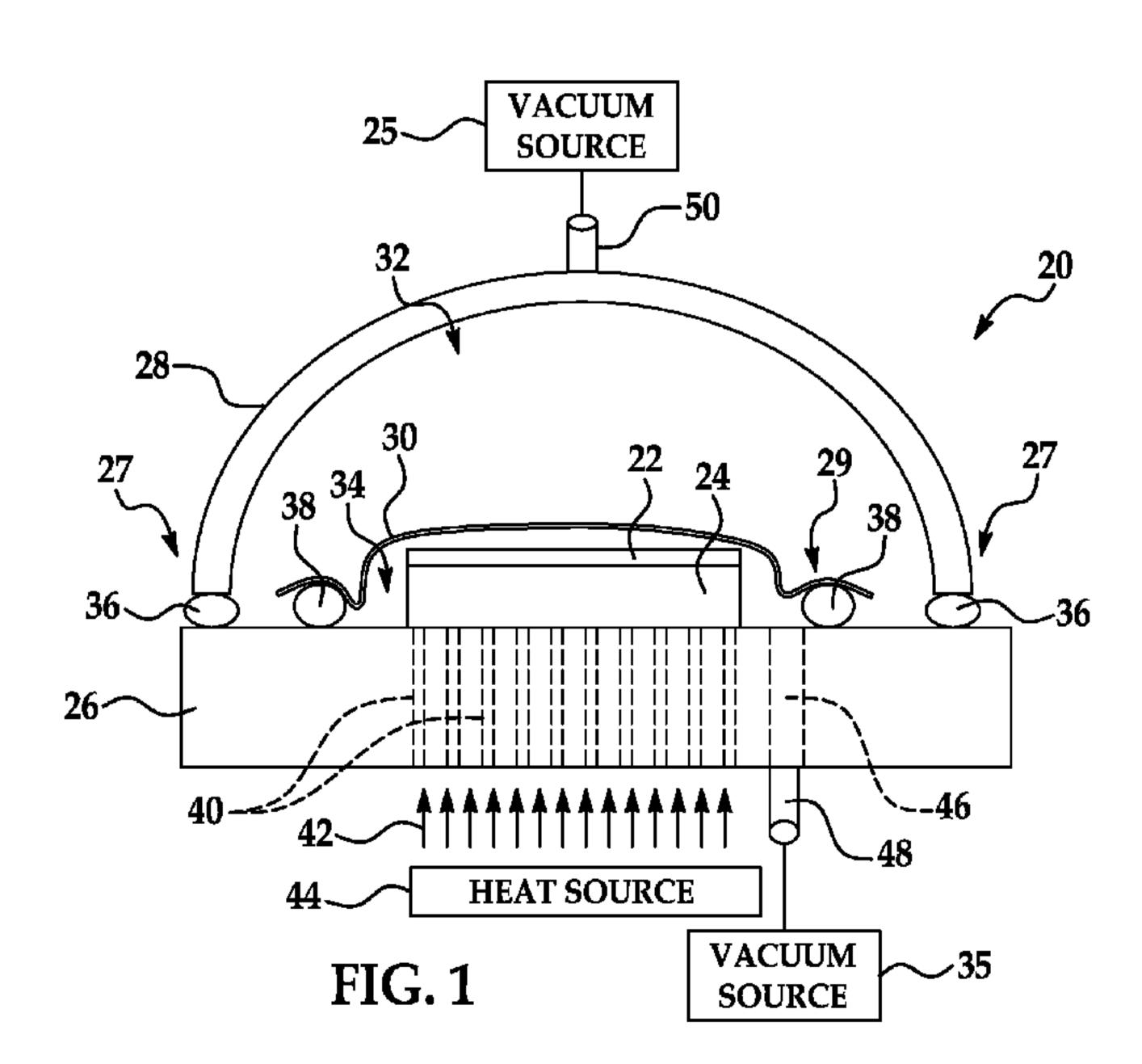
(57) Abstract: Out-of-autoclave curing of a composite part is performed using a double vacuum chamber assembly comprising integrated inner and outer vacuum chambers.
