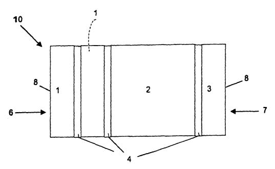
(57) Abstract: Transparent panels having unidirectional bullet-resisting characteristics contain at least one sheet of glass, several intermediate sheets formed of an acrylic resin or further glass sheets, and an inner sheet formed of a polycarbonate resin. A transparent adhesive bonds the sheets to each other to form the panel. The level of bullet resistance capability is measured according to NIJ standards and the panels have a Level III or Level IV rating.
