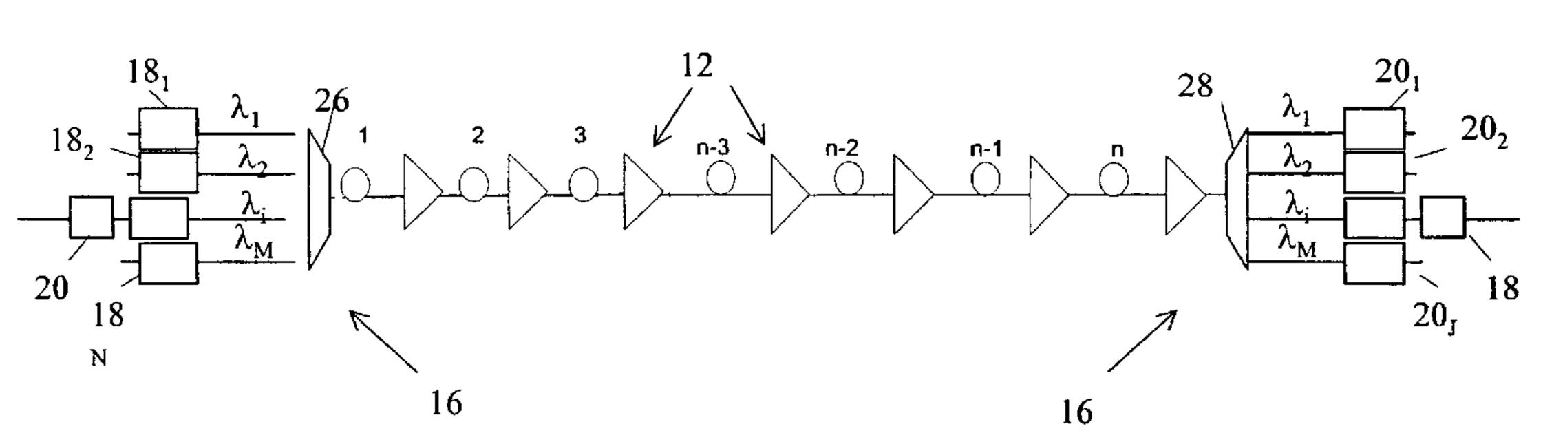
(57) Abstract: Optical transmission systems of the present invention include a plurality of optical amplifiers configured to provide optical amplification of one or more information carrying optical signal wavelengths. At least two of the optical amplifier are operated to provide net losses or net gains along corresponding spans, while the cumulative gain provided by the plurality of optical amplifiers substantially compensates for the cumulative loss of the spans.
