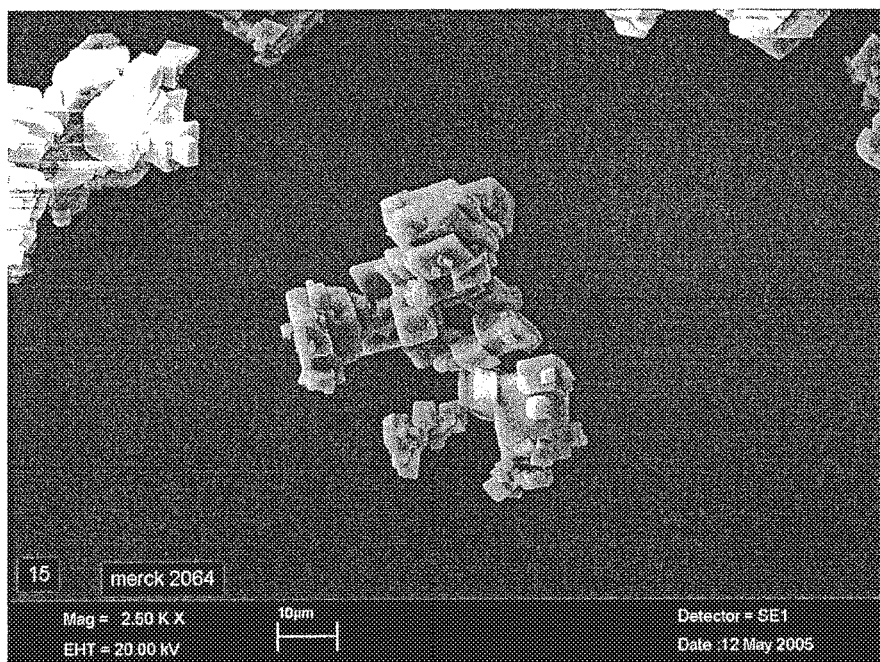
Agglomerate of regular shaped calcium carbonate Merck 2064 crystals
