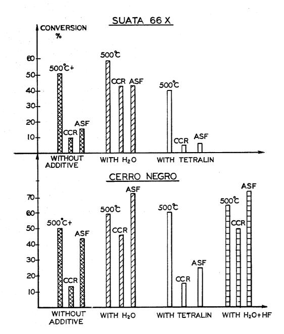
REACTOR SOAKER 430°C, 127 ATM, 1.55h EFFECT OF ADDITIVES IN VARIATIONS OF PROPERTIES.
