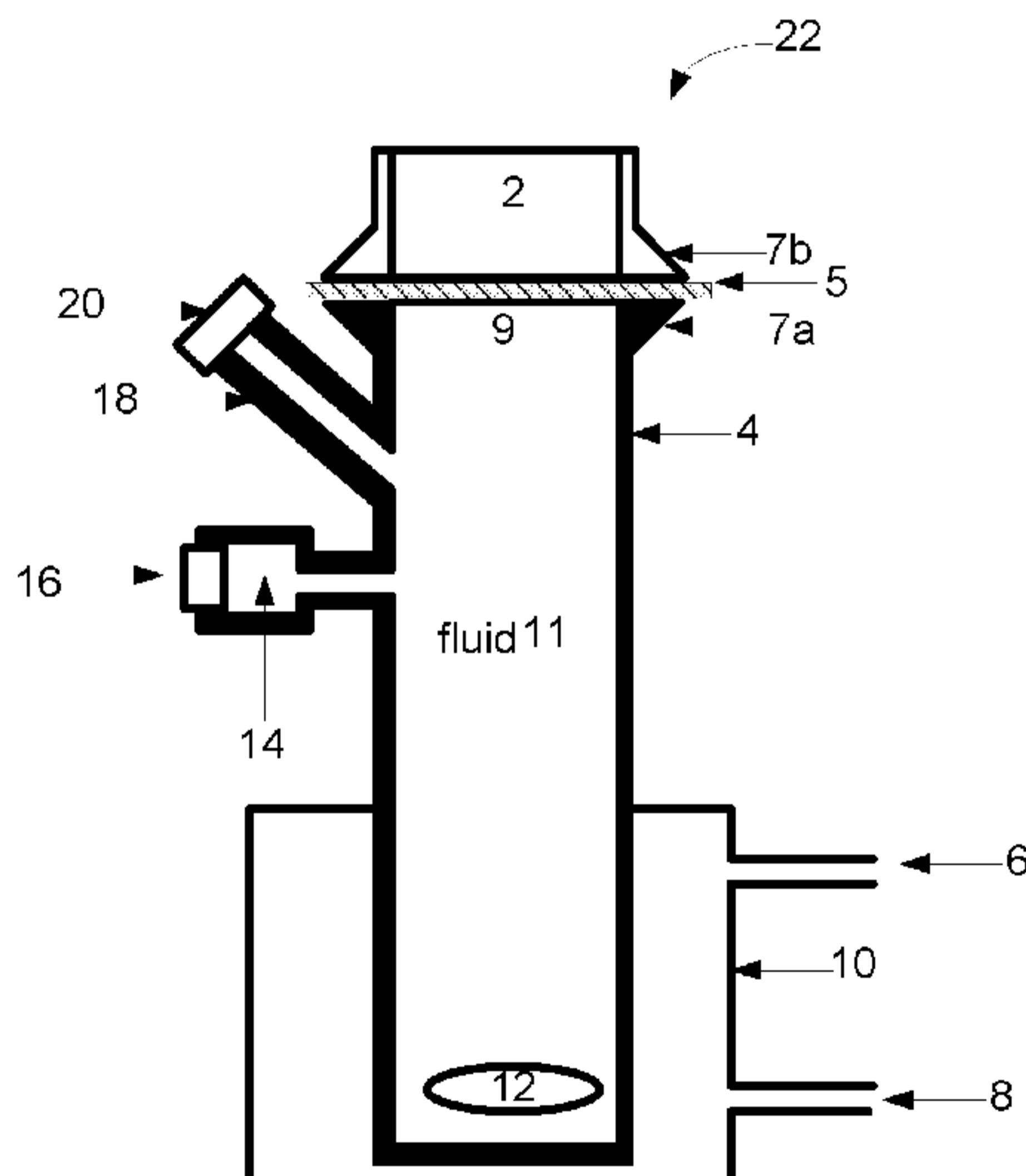
(57) Abstract: A skin sample is mounted in a diffusion cell between a receptor and a donor chamber. A substance to be tested is provided to the skin sample via the donor chamber. The diffusion cell has a driver for applying pressure variations to fluid in the receptor chamber in order to cause repeated flexing of the skin sample to simulate the behaviour of living (moving) skin.
