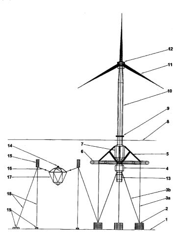
(57) Abstract: The invention is related to a method of positioning chains or pipes on the upper part of a floating foundation in order to make the foundation more rigid and stable.
