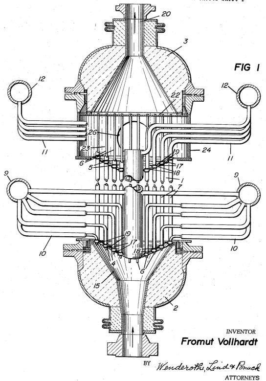
HEAT EXCHANGER FOR COOLING CRACKED GASES BY MULTIPLE MEDIA
