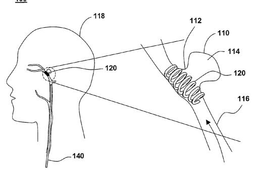
(57) Abstract: The present invention provides a system for treating an aneurysm, including a catheter with a stent receiving tube and coiled stent axially received in the stent-receiving tube, wherein the coiled stent is delivered to the aneursym through a vessel via a catheter. The present invention also provides a coiled stent and a method of treating an intracranial aneurysm.
