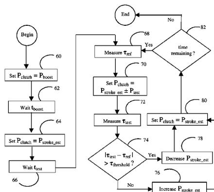
method includes varying the fluid pressure around a predetermined value, measuring a resulting torque difference with the torque sensor, and adjusting a clutch control parameter if the resulting torque difference is less than a threshold value.
