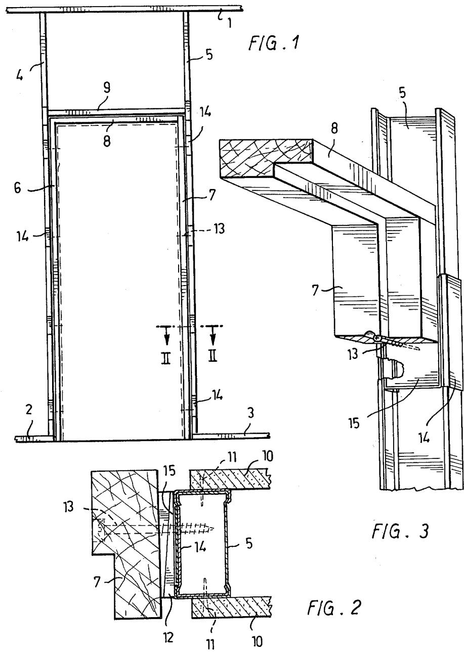
MEANS FOR FASTENING A FRAME TO A WALL
