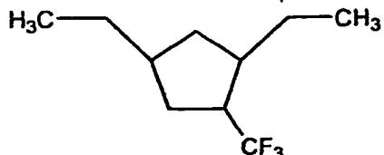
10 (Molecular model in which both ends of a repeated structural unit of the formula (1) wherein R<sup>2</sup> is CF<sub>3</sub>, X<sup>1</sup> is CH<sub>2</sub>, the others are each hydrogen, and n is 0 are capped with methyl groups in a hydrogenated polymer of a ring-opening metathesis polymer.)
