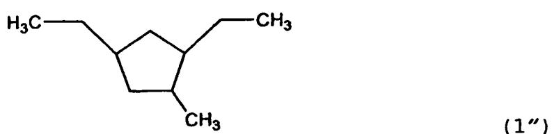
25 (Molecular model in which both ends of a repeated structural unit of the formula (1) wherein R<sup>2</sup> is CF<sub>3</sub>, X<sup>1</sup> is CH<sub>2</sub>, the others are each hydrogen, and n is 0 are capped with methyl groups, and fluorine is replaced with hydrogen in a hydrogenated polymer of a ring-opening metathesis polymer.)
