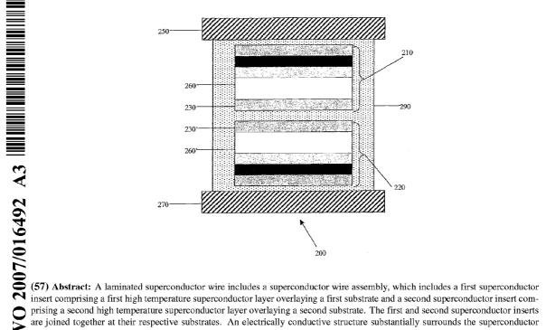
are joined together at their respective substrates. An electrically conductive structure substantially surrounds the superconductor wire assembly
