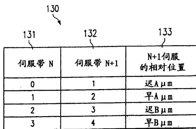
Diagram illustrating the relative positions of servo tapes N and N+1. The top row shows the servo tape numbers: 130, 131, 132, and 133. Brackets group 131 and 132 as '伺服带 N+1' (Servo Tape N+1), and 132 and 133 as 'N+1伺服的相对位置' (Relative Position of N+1 Servo). The bottom part is a table:
