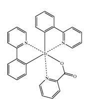
which differ from the compounds of the formula (I) by replacement of a phenylpyridine ligand by a pyridine-2-carboxylic acid ligand, can be used as the electrophosphorescent compound.
