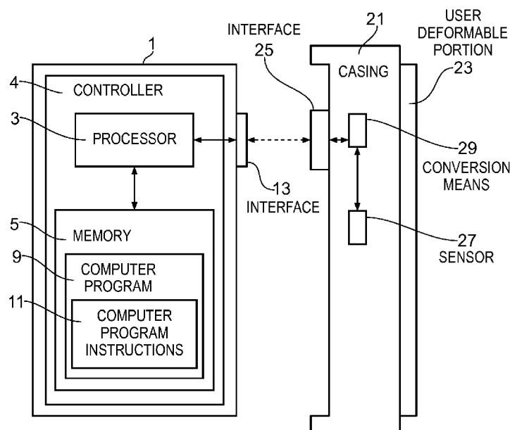
(57) Abstract: A casing, method and apparatus wherein the casing comprises: at least one user deformable portion; at least one sensor configured to detect deformation of the at least one user deformable portion; wherein the casing is configured to be removably coupled to an apparatus and is configured so that, in response to detecting the deformation of the user deformable portion of the casing, a control signal for control of the apparatus is provided.
