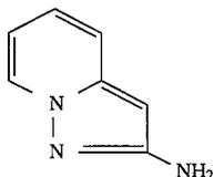
2.66 g. 2-Aminopyrazolo[1,5-a]pyridine (see Chem. Pharm. Bull., 21, 2146/1973) are reacted with p-methoxybenzenediazonium salt analogously to Example 12.3.1, the resultant azo compound is reduced with sodium dithionite and the crude product obtained is purified to give 2,3-diaminopyrazolo[1,5-a]pyridine; m.p. 190° C.;  $R_f=0.6$  (silica gel, ligroin/acetone/glacial acetic acid 60:40:1 v/v/v).
