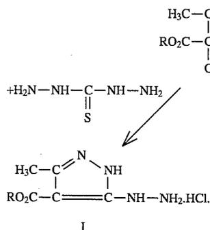
For the synthesis of 4-ethoxy carbonyl-3-methyl-pyrazolo-5-yl-hydrazine 10.6 g thiocarbonylhydrazide ( $\text{H}_2\text{N}=\text{NH}=\text{CSNHNH}_2$ ) are suspended in 100 ccm of ethanol and 30 ccm hydrochloric acid are added while boiling. Under stirring 16.5 g ethyl  $\alpha$ -chloro-acetoacetate dissolved in 20 ccm ethanol are added dropwise within 30 minutes. After cooling a crystal mask of the product separates which can be recrystallized from ethanol.
