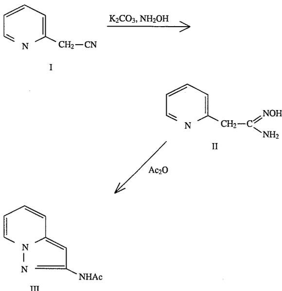
Compound II, prepared from pyridine-2-acetonitrile (I) and hydroxylamine, was treated with excess acetic anhydride at  $100^\circ C$ . for 30 minutes and the reaction products were separated by chromatography on alumina.
