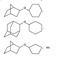
It is part of my invention that ether oxygenates enhance cleaner burning properties and elevate cetane number by <sup>40</sup> their ability to initiate radical processes essential for efficient combustion. This is affected in part by their ability to form peroxides which then act as radical sources. This effect can be enhanced by storing the diesel fuel ether supplement blends in contact with oxygen or air or by passing oxygen or <sup>45</sup> air through them.
