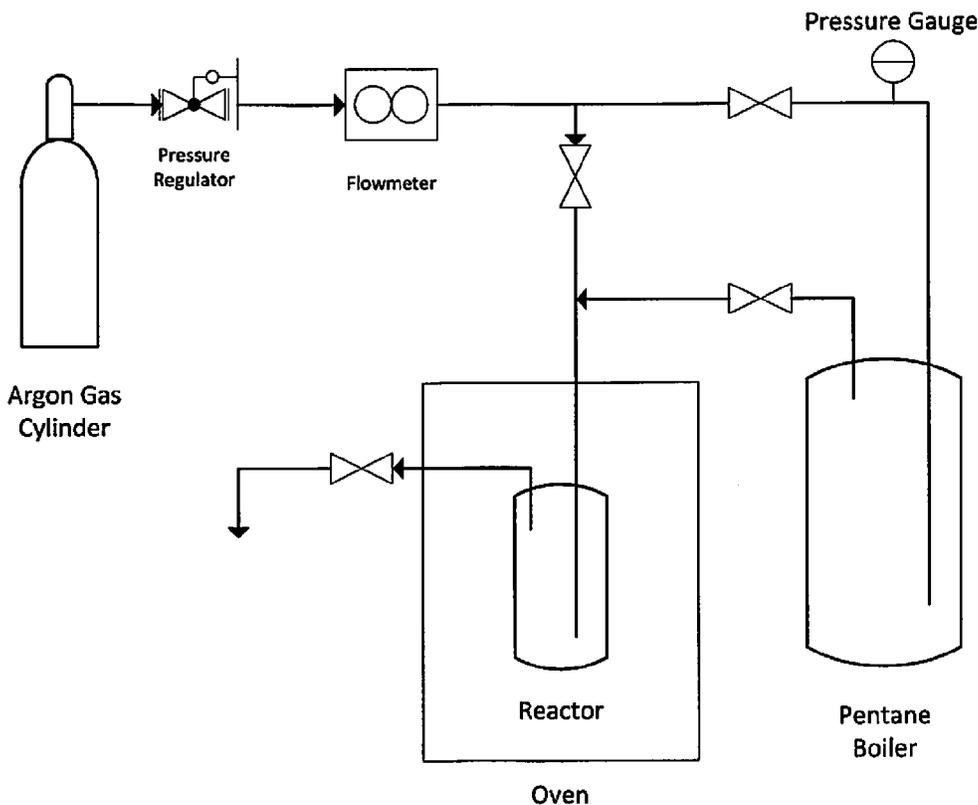
**Diagram of magnesium carbide reactor set up**
