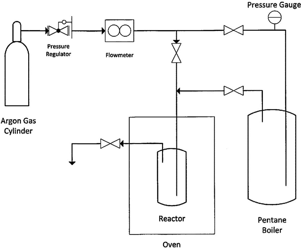
Figure 1. Diagram of magnesium carbide reactor set up
