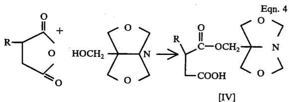
can be employed to catalyze the esterification process. In general, the reaction is effected in a reactor in the absence of or presence of an inert diluent such as xylene and solvent oil and heating the mixture from about 50° C. to about 230° C. preferably 70° C. to 150° C. for about 10 minutes to 48 hours, more preferably 1 to 3 hours. Completion of reaction can be readily discerned by infrared analysis.
