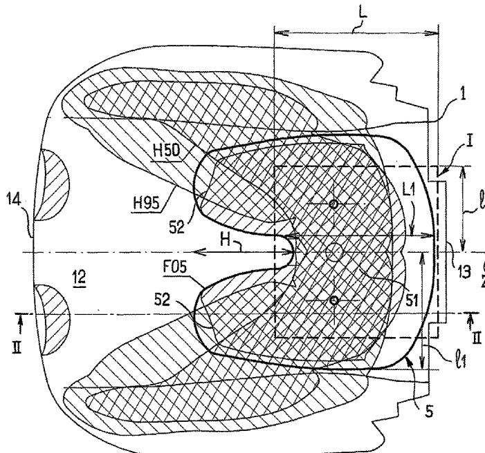
(57) Abstract: The invention relates to a base cushion (1) for a motor vehicle seat, comprising a body (11), made from elastomeric foam, the seating face (12) of which has a recess (3). The invention is characterised in that a support element (5), comprising at least one pocket filled with a viscoelastic gel is placed in the recess (4) such as to come into contact with the ischiatic region of a user seated on said cushion (1).
