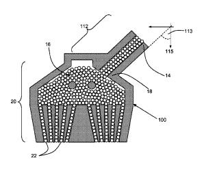
end of the stacking channel, and distributing the plurality of rod-shaped consumer goods from the hopper into a packing apparatus.
