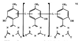
which contain one or more resorcinol derived moieties have UV spectra which are red-shifted to the near UV range and provide excellent stabilization to polymeric substrates against the deleterious effects of actinic light.
