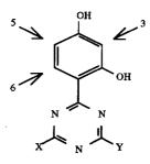
U.S. Pat. Nos. 3,118,887 and 3,268,474 describe the protection of plastic and resinous compositions from UV light by the incorporation of one or more compounds of the class of tris-aryl-s-triazines. The former patent claims 2,4, 35 6-tris-(2,4-dihydroxyphenyl)-s-triazine and 2,4,6-tris-(2hydroxy-4-alkoxyphenyl)-s-triazines. A tris-5alkylresorcinol-s-triazine is prepared, but not tested or claimed.
