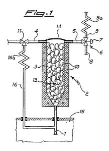
This invention relates to a process and a relevant device for the introduction of liquid samples into apparatuses for gas chromatographic analysis, specially designed for samples containing high percentages of solvent and namely samples having relatively large volume, containing compounds to be analysed in very low concentrations in the relevant solvent.
