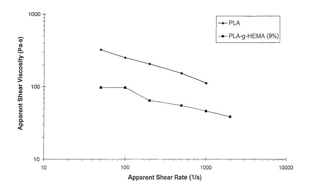
Figure 1. Melt Rheology at 180°C for PLA and HEMA Grafted PLA
