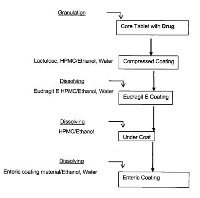
Manufacturing Flow of the Colon-Targeted Tablet
