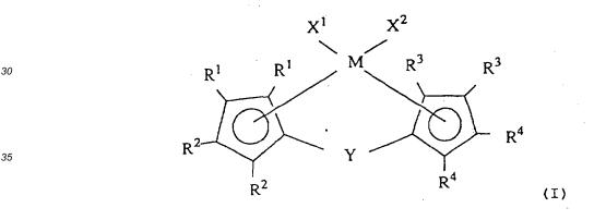
40 wherein M is a transition metal atom of Group 4 to Group 6 of the periodic table, specifically titanium, zirconium, hafnium, vanadium, niobium, tantalum, chromium, molybdenum or tungsten, preferably titanium, zirconium or hafnium, particularly preferably zirconium.
