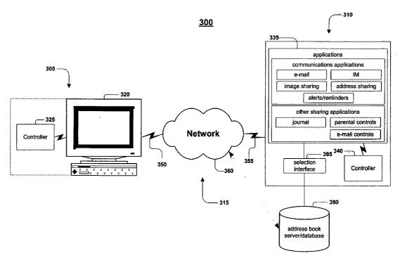
(57) Abstract: Enabling management of contacts includes creating a single list of contacts that is stored in a central repository (380). A member (305) is enabled to define a group of contacts from the single list of contacts and represent the group of contacts by a unique identifier (430). The member is enabled to adress communications sent from multiple applications to the group of contacts represented by the unique identifier.
