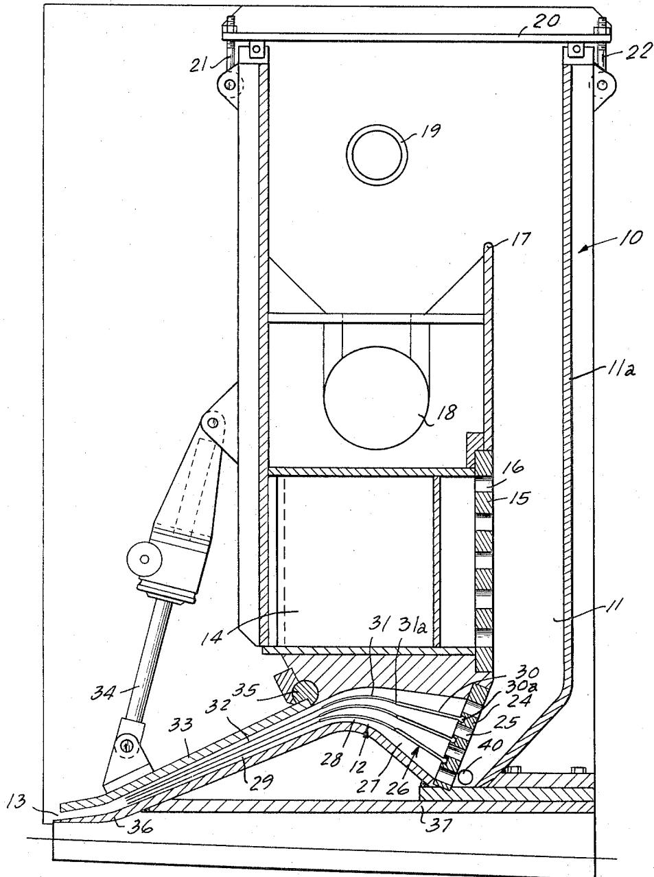
**PAPERMAKING MACHINE HEADBOX WITH AN UPWARDLY INCLINED SLICE CHAMBER PORTION, AN ARCUATE PORTION, AND A DOWNWARDLY INCLINED PORTION AND CONTAINING FLEXIBLE TRAILING MEMBERS**
