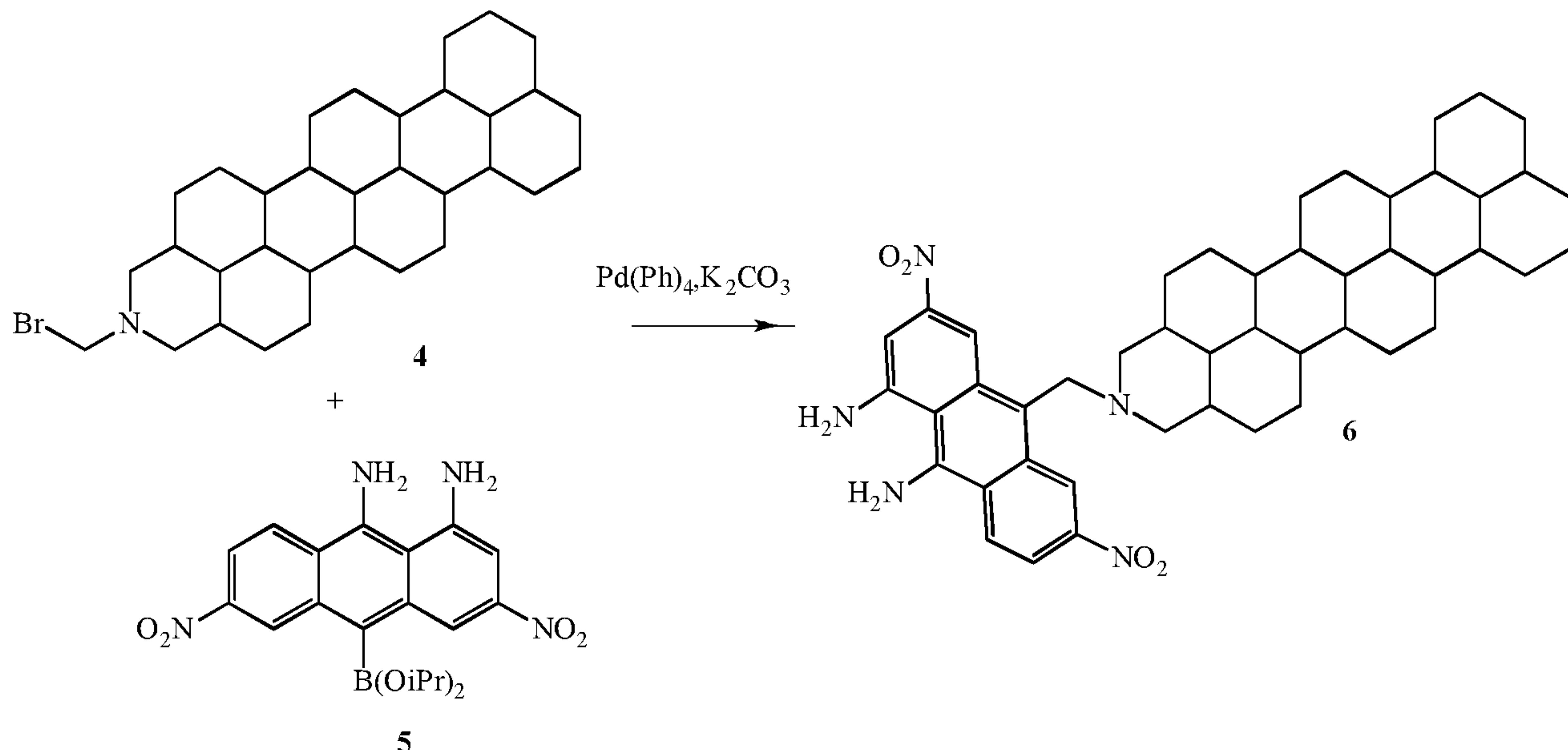
Bromo-amine **4** (1 equiv.), Anthracene **5** (1 equiv.),  $\text{Pd}(\text{Ph})_4$  (10 mol %),  $\text{K}_2\text{CO}_3$  (1.5 equiv.) were stirred in toluene at 70 °C for 18 h. The mixture was filtered through Celite and the filtrate was washed with  $\text{NaHCO}_3$  and brine. The organics were dried over  $\text{MgSO}_4$ , and the solvents were removed under reduced pressure to give **6**.
