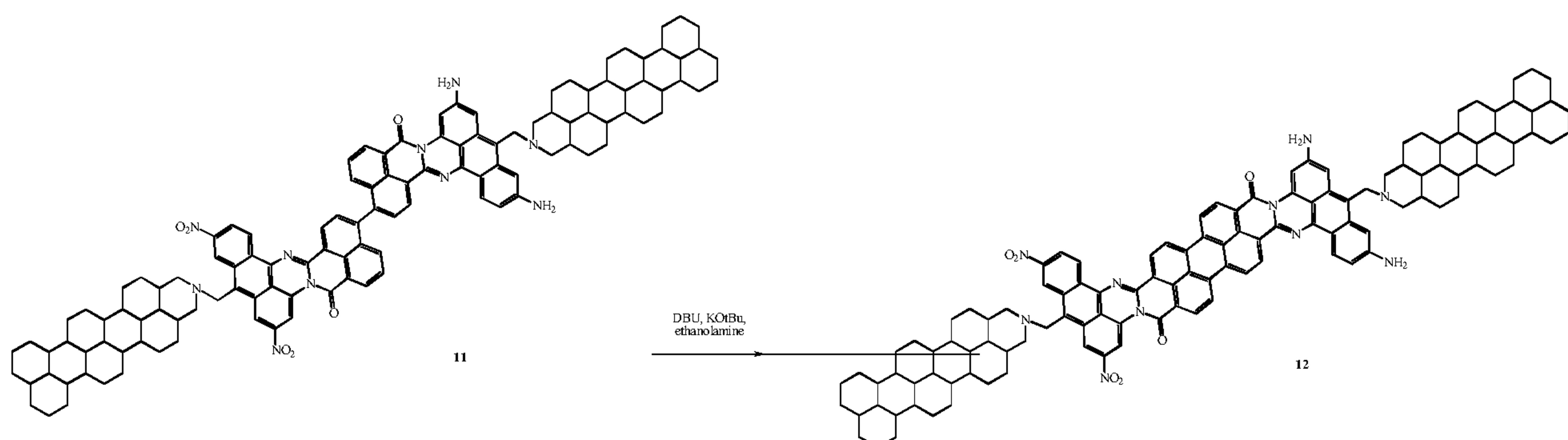
A mixture of 1.48 g (13 mmol) potassium tert-butoxide 2.30 g (15.1 mmol) of diazabicyclo[5.4.0]undec-7-ene (DBU), 2.2 g 36.3 mmol) ethanolamine and 1.0 g of **11** was heated to 140 °C for 11 hours. Afterwards, the same amount of potassium tert-butoxide, DBU and ethanolamine were added and the mixture was kept at 140 °C for 18 hours. The reaction mixture was cooled to room temperature, poured into 250 ml of 1M HCl filtered, washed until neutral pH and then dried to give the final product **12**.
