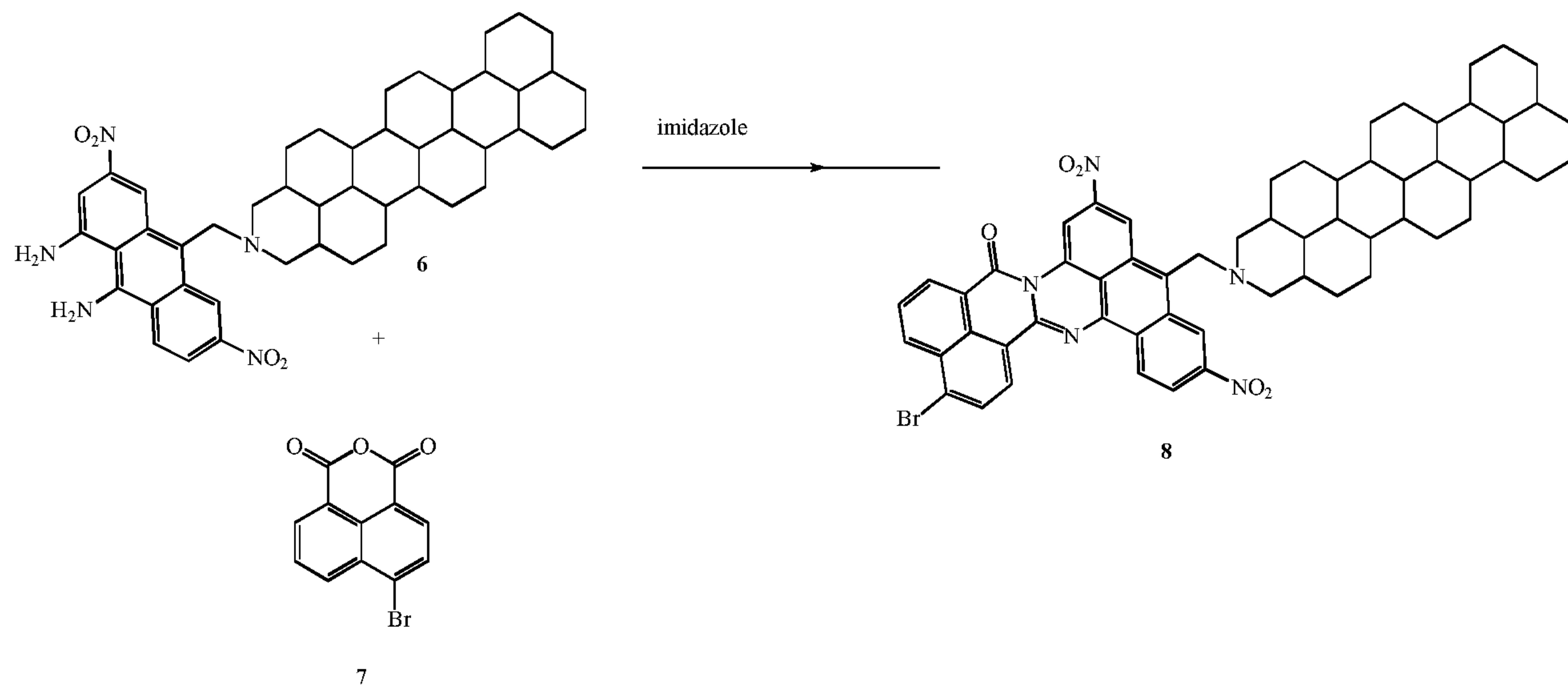
Naphthalene anhydride **7** (1 equiv.) and anthracene **6** (1 equiv.) were stirred in imidazole at 130 °C overnight. The mixture was dissolved in THF and washed with water 3 times. The
