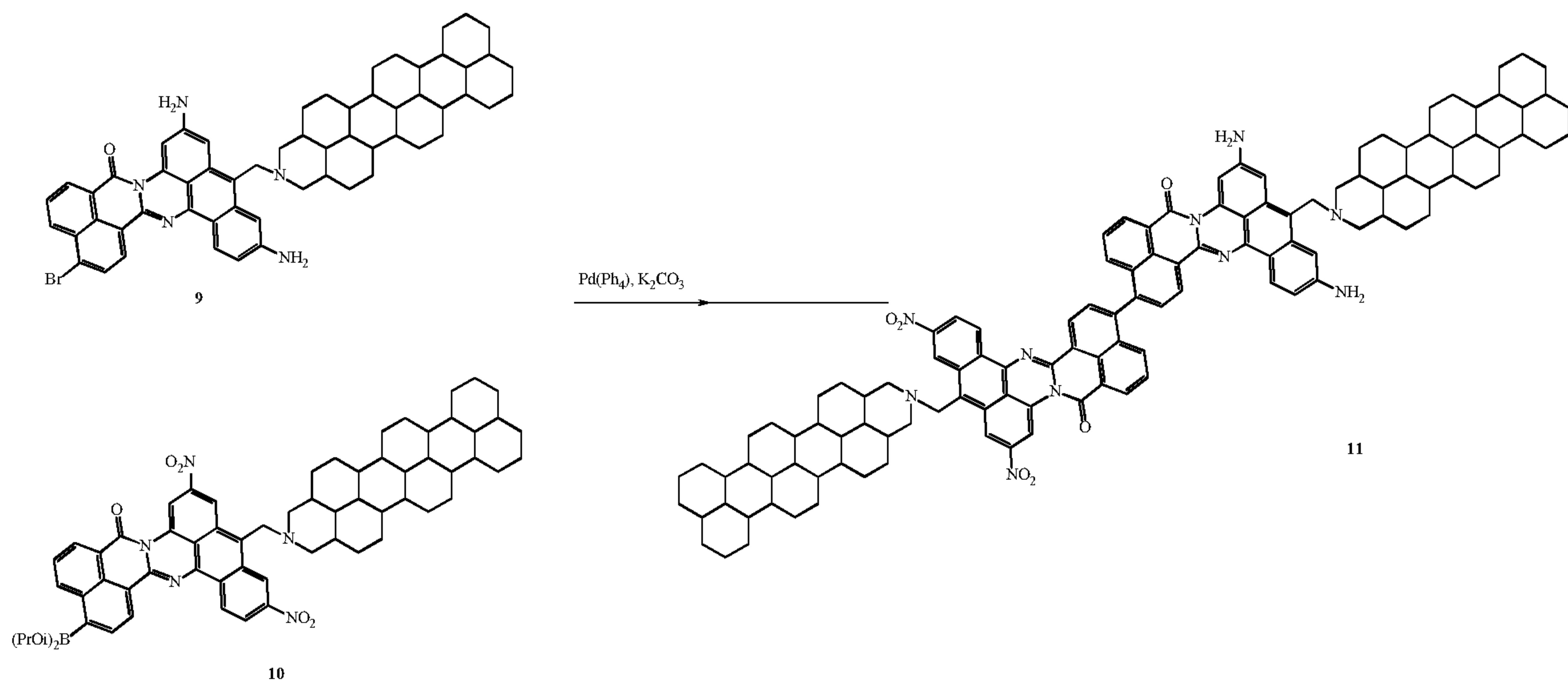
Bromo-amidine **9** (1 equiv.), Amidine boronic ester **10** (1 equiv.),  $\text{Pd}(\text{Ph}_4)$  (10 mol %),  $\text{K}_2\text{CO}_3$  (1.5 equiv.) were stirred in toluene at 70 °C for 18 h. The mixture was filtered through Celite and the filtrate was washed with  $\text{NaHCO}_3$  and brine. The organics were dried over  $\text{MgSO}_4$ , and the solvents were removed under reduced pressure to give **11**.
