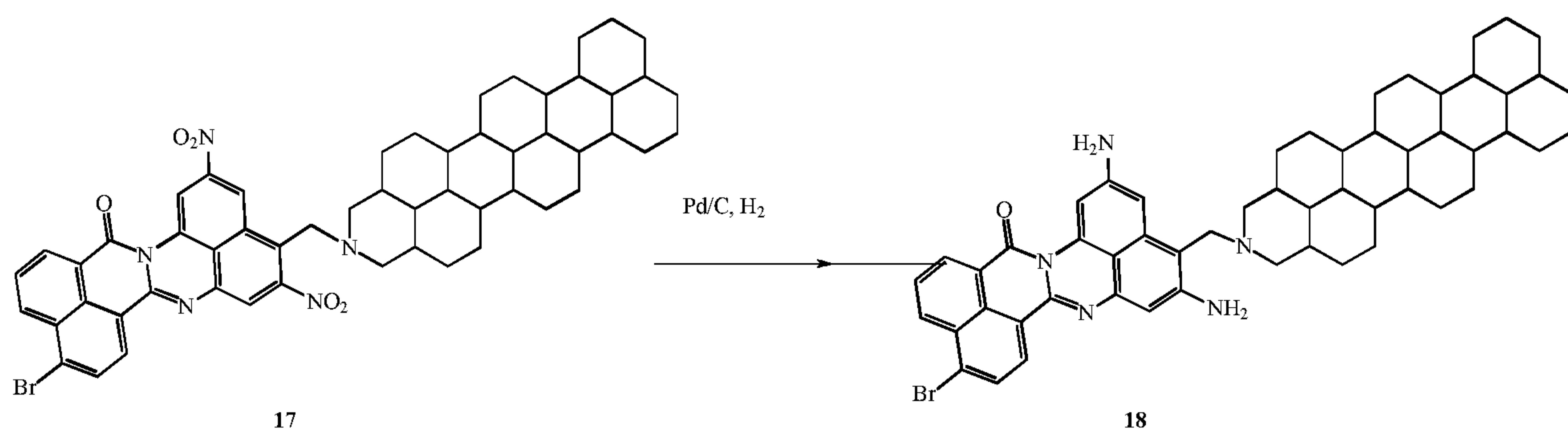
Amidine **17** (1 equiv.) and Pd/C (20% wt/wt) were stirred in THF in a three-neck flask with a H<sub>2</sub> balloon attached for 18 h. The mixture was filtered through Celite and the solvents were removed under reduced pressure to give **18**.
