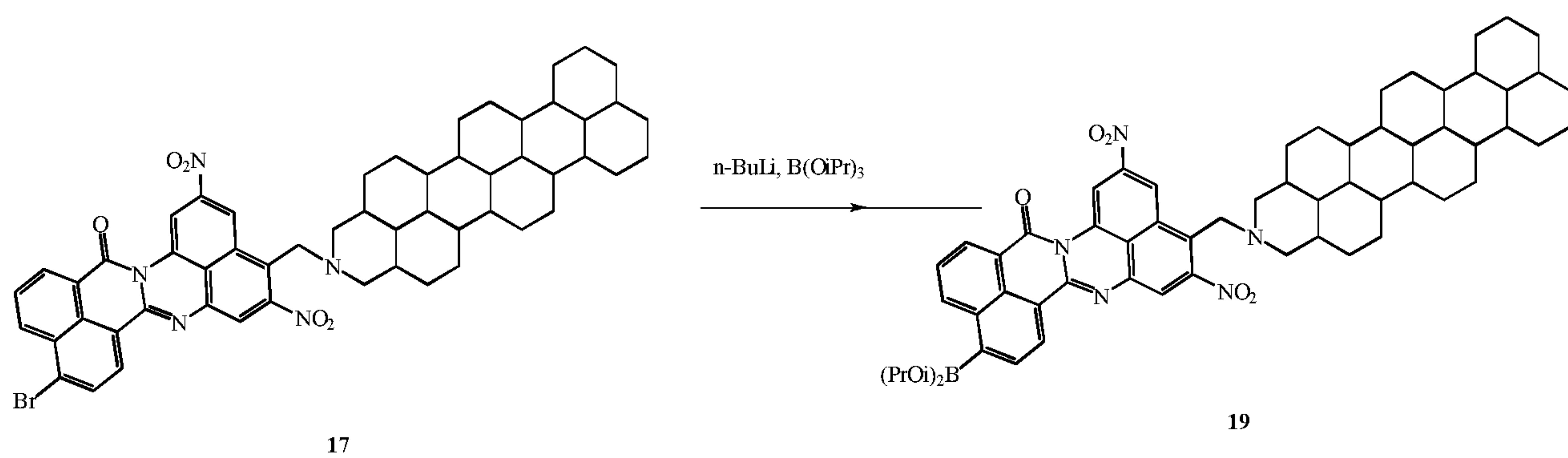
Amidine **17** (1 equiv.) was dissolved in THF and stirred at  $-80^{\circ}\text{C}$ . N-butyllithium (1.2 equiv., 2.5 M in hexanes) was added dropwise. After 1 h, triisopropylborane was added dropwise and allow to warm to room temperature overnight. The mixture was washed with  $\text{NaHCO}_3$  and brine and dried over  $\text{MgSO}_4$ . The solvent was removed under reduced pressure to give **19**.
