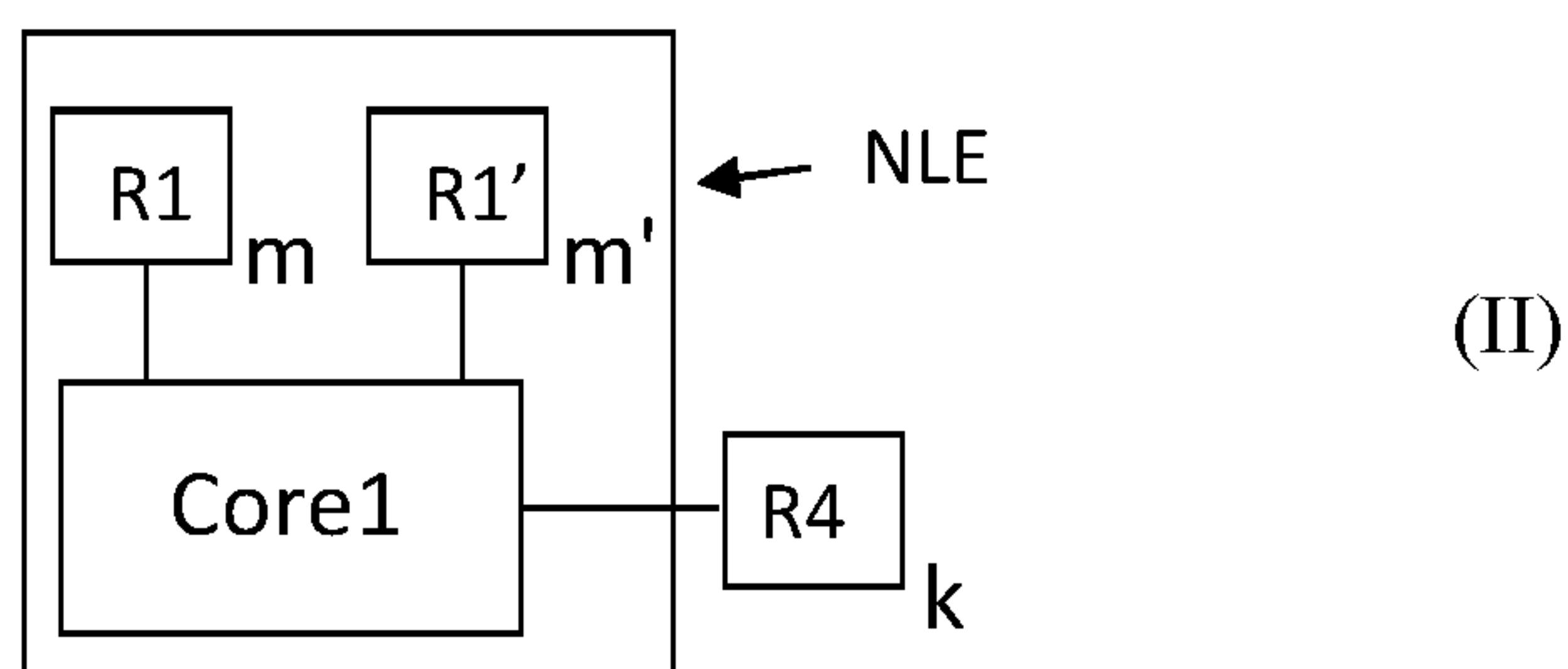
wherein the Core1 is the aromatic polycyclic conjugated molecule, resistive substituents R4 are a non-conjugated part of compound II, and are either monocycles or fused polycycles, wherein the monocycles or polycycles are either saturated hydrocarbons or saturated halocarbons forming rigid spatial structures with dense packing of SP3 carbon saturated with H, F, Cl, and/or Br, and
