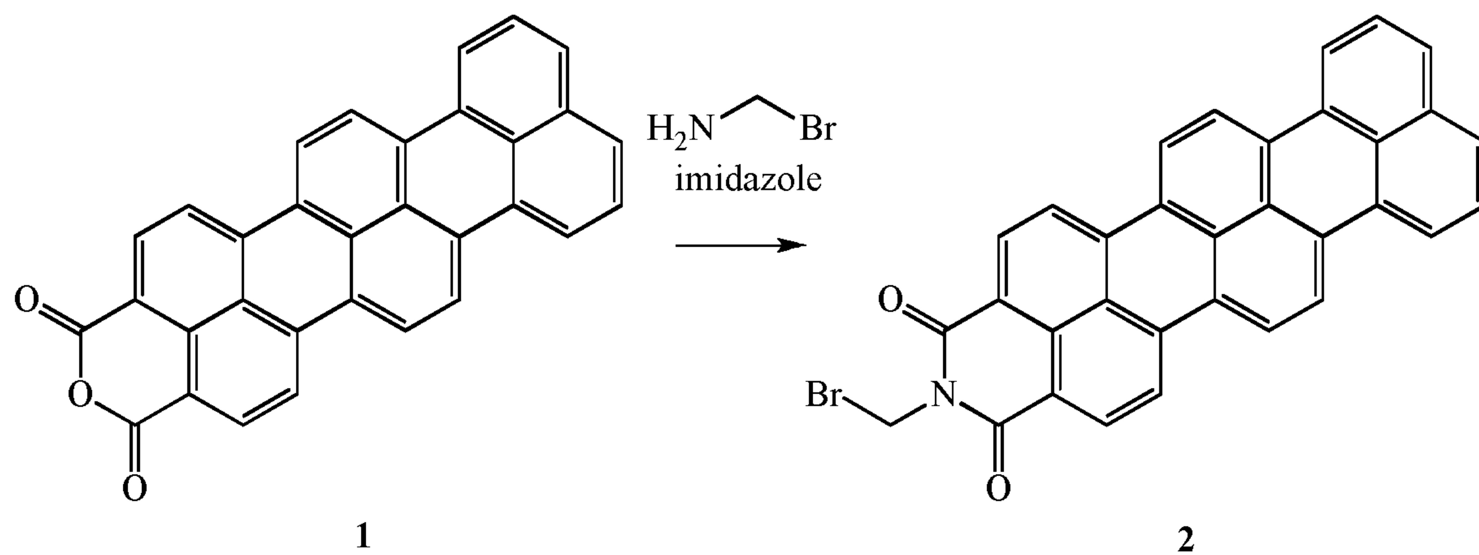
Terrylene anhydride **1** (1 equiv.) and 1-bromomethanamine (1 equiv.) were stirred in imidazole at 130 °C overnight. The mixture was dissolved in THF and washed with water 3 times. The
