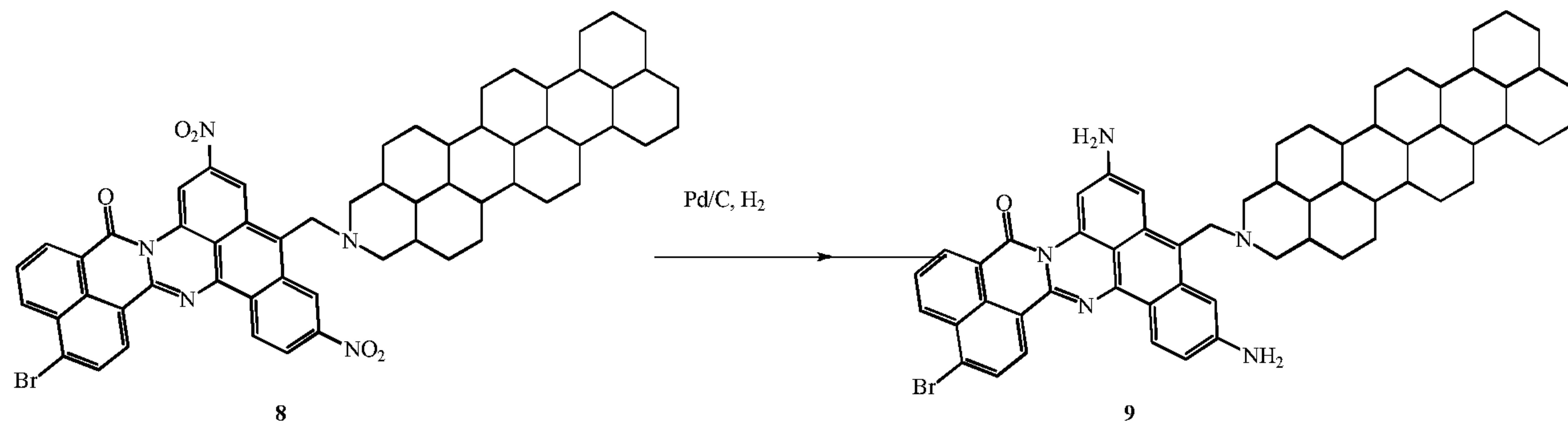
Amidine **8** (1 equiv.) and Pd/C (20% wt/wt) were stirred in THF in a three-neck flask with a  $\text{H}_2$  balloon attached for 18 h. The mixture was filtered through Celite and the solvents were removed under reduced pressure to give **9**.
