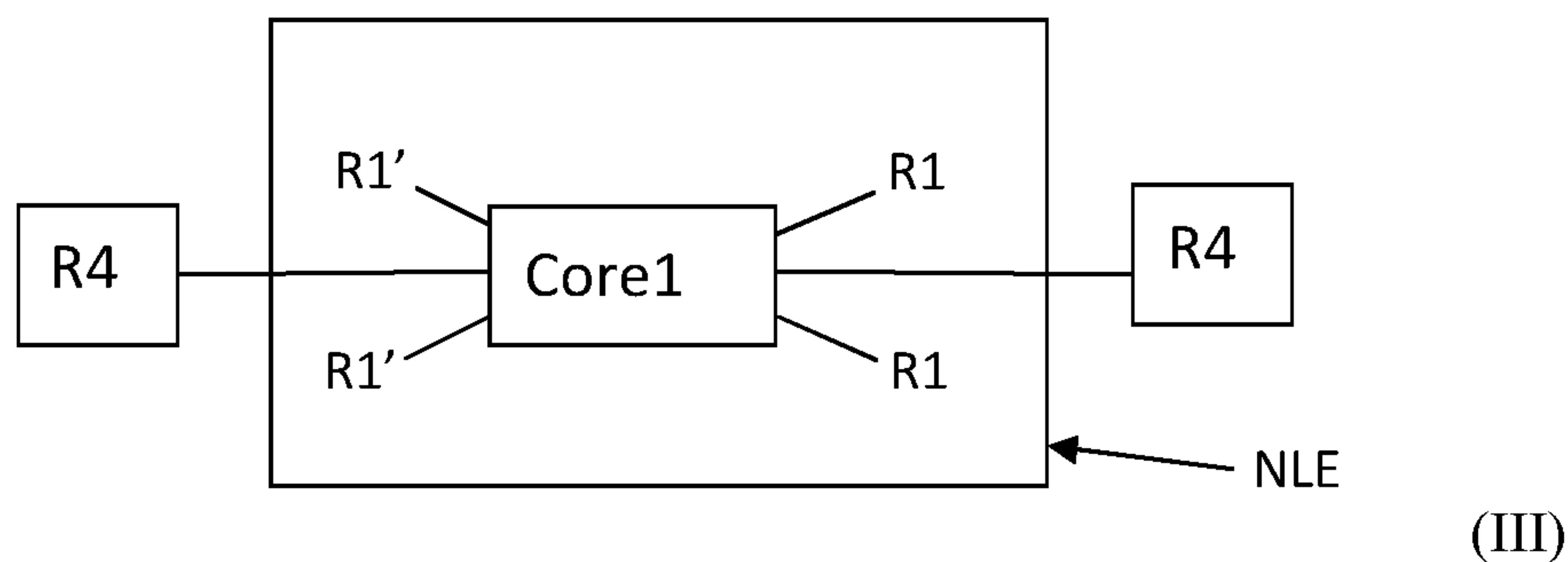
In general formula III, the parameter  $m$  is equal to 4,  $R1'$  is donor group,  $R1$  is acceptor group,  $k$  is equal to 2. In another embodiment of the electro-polarizable compound, the Core1 is rylene fragment having following structural formula where repetition parameter  $t$  is an integer varying from 0 to 5:
