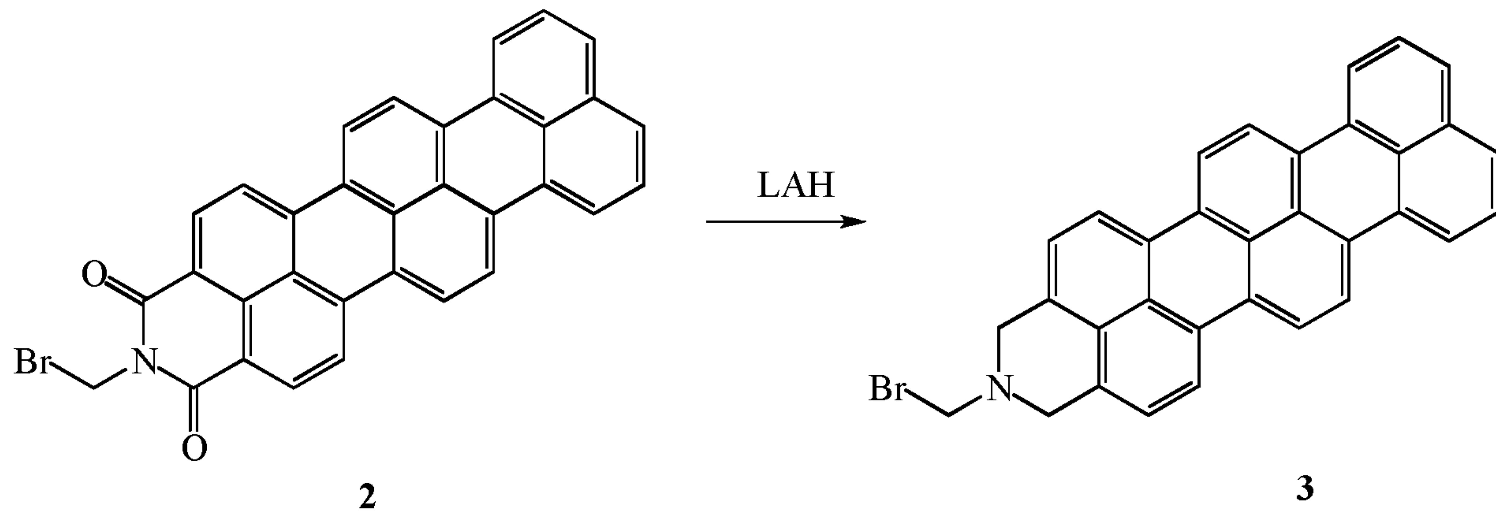
Terrylene imide **2** (1 equiv.) was dissolved in THF and stirred over an ice bath. Lithium aluminum hydride (5 equiv.) dissolved in THF was slowly added. The mixture was allowed to warm to ambient temperature and stirred for 18 h. The mixture was quenched with 2M NaOH, filtered, and dried over  $\text{MgSO}_4$ , and the solvent was removed under reduced pressure to give **3**.
