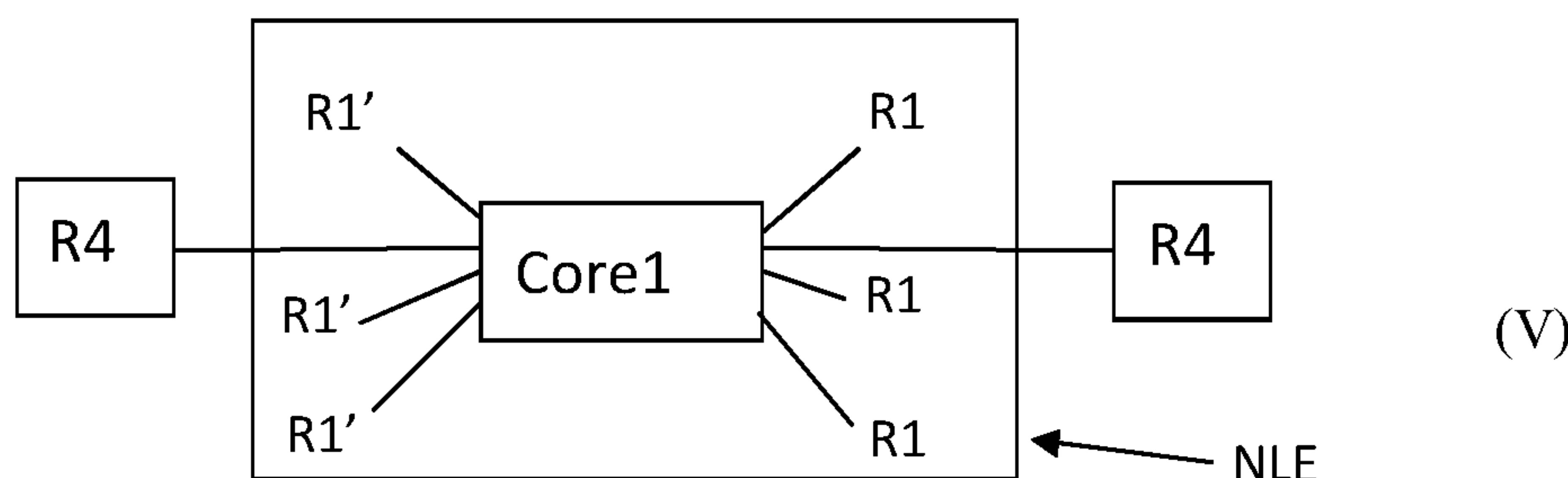
In general formula V, Core1 is the above-described aromatic polycyclic conjugated molecule,  $m$  is equal to 6,  $R1'$  is donor group,  $R1$  is acceptor group,  $k$  is equal to 2. In yet another embodiment of the electro-polarizable compound, the Core1 is rylene fragment having following structural formula where repetition parameter  $t$  varies from 1 to 5:
