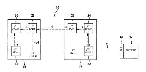
(16) if interference is detected by means of the first control unit (14) and/or the second control unit (16). The invention makes possible spatial separation of the control unit to be tested from the control unit carrying out the switching off, wherein the installation position of the control unit to be tested can be selected freely.
