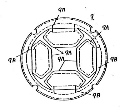
9....sealing part 9A...dlaphragm 9B...penetrating hole
