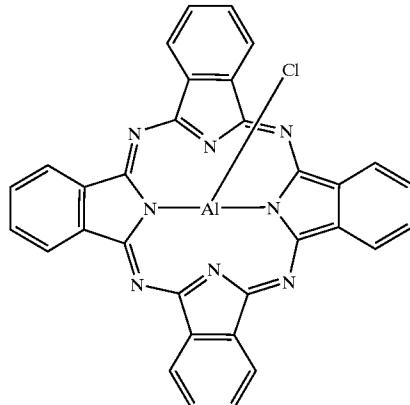
[0328] The dye monochloro-aluminium-phthalocyanine (AlClIPc) was applied for the information layer. The disc structure employed was as shown in **FIG. 2a**.
