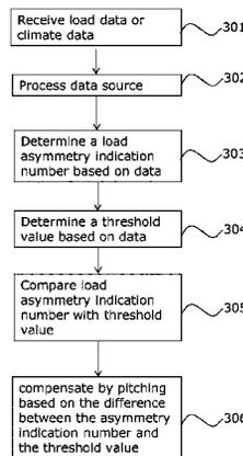
loading of the wind turbine or based on climate conditions under which the turbine operates.
