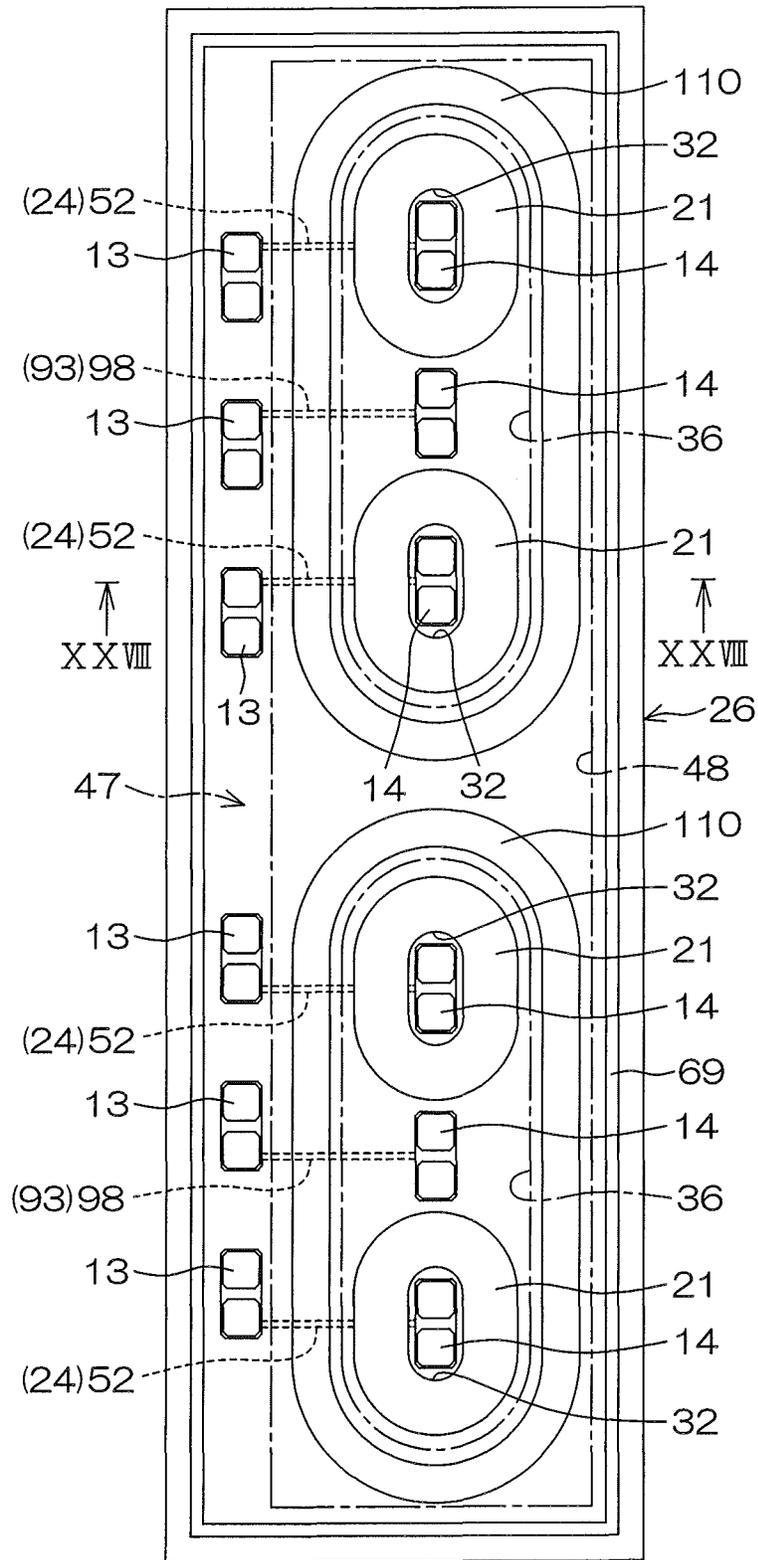
FIG. 26 (LOWER COIL PLANE)
