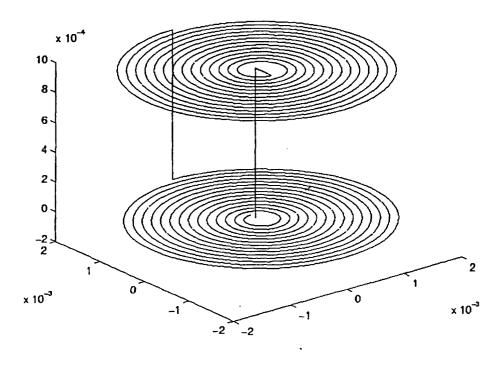
Figure 1: The microcoil configuration with a single pair of radially-opposed spirals. The z-axis points upward in this plot.
