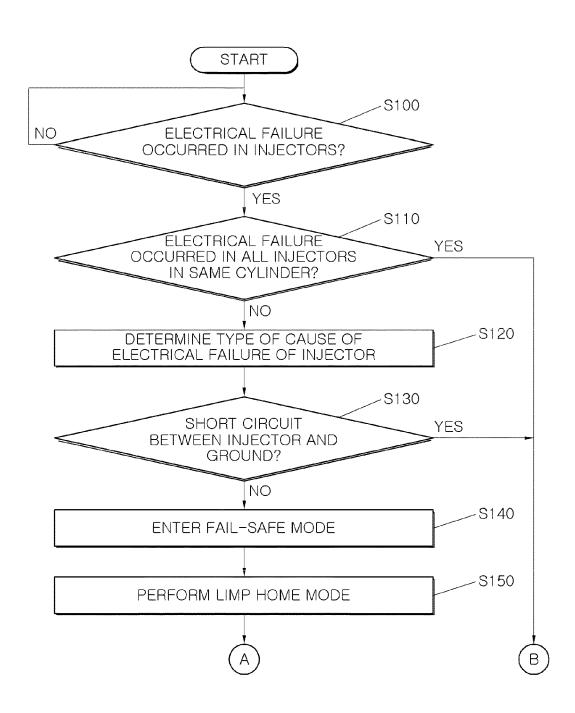
\$180 CUT OFF FUEL SUPPLY TO ALL INJECTORS IN SAME CYLINDER 9 S170 S160 CUT OFF FUEL SUPPLY TO ABNORMAL INJECTOR REQUIRED TOTAL FUEL AMOUNT < INJECTABLE FLOW RATE OF ONE INJECTOR? IN SAME CYLINDER, AND INCREASE AMOUNT OF FUEL INJECTFDBY NORMAL INJECTOR END ⋖
