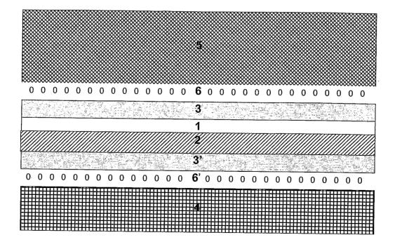
(57) Abstract: Chitosan films and laminates made from the films are provided. The films and laminates can be used to make a variety of finished articles that can be used to provide protection from hazardous chemical and biological agents.
