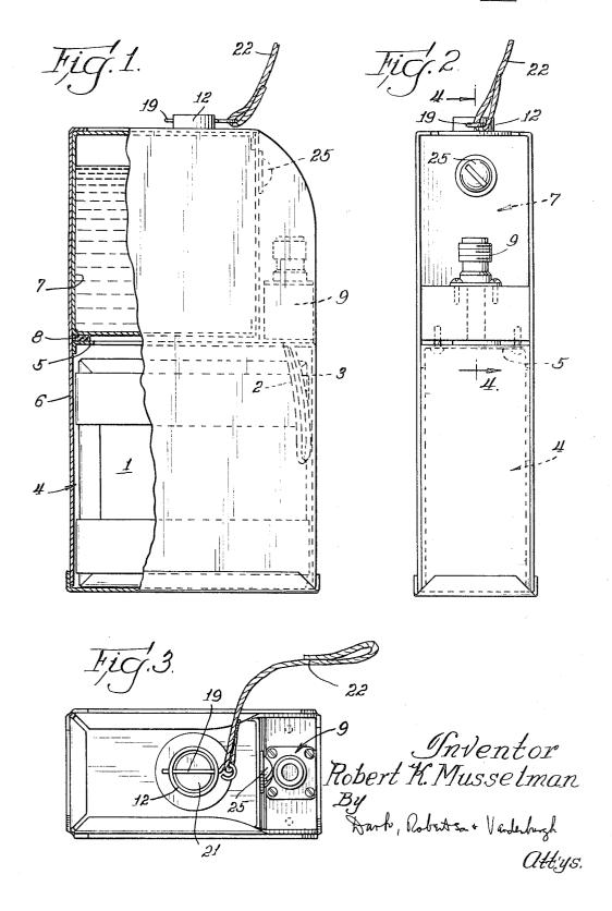
ELECTROLYTE RELEASE VALVE AND VENT FOR RESERVE BATTERY Filed Nov. 7, 1966 Sheet 2 of 2 23 27-18 8 Inventor
