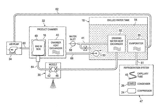
(57) Abstract: A system and method for dispensing fluids is introduced. A preferred embodiment comprises a sealed tank, a bag containing fluid inside the sealed tank, an outlet for dispensing the liquid in the bag, and a pressure generating device to create pressure in the sealed tank.
