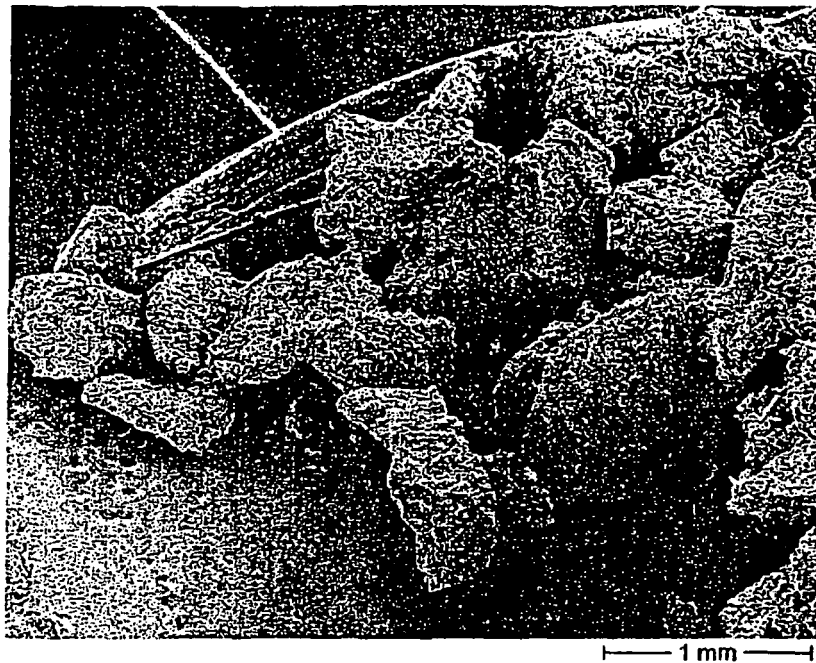
Figure 13B: Surface of Nal-Extr granulates at 200x magnification. The voltage was 10 kV. The bar length corresponds to 100 \mu m.
