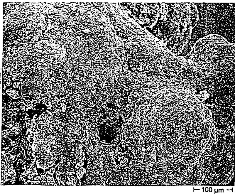
Figure 12B: Surface of Nal-10-Sure granulates at 200x magnification. The voltage was 10 kV. The bar length corresponds to 100 \mu m.
