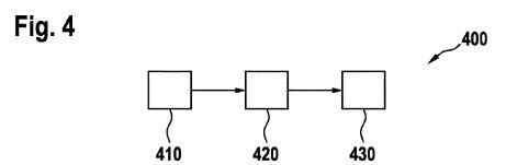
410 FIRST STEP - INFORMATION RECEIVED BY EVALUATION UNIT 420 SECOND STEP - EVALUATE INFORMATION TO GENERATE CONTROL INFORMATION 430 THIRD STEP - SEND CONTROL INFORMATION TO CONTROL UNIT
