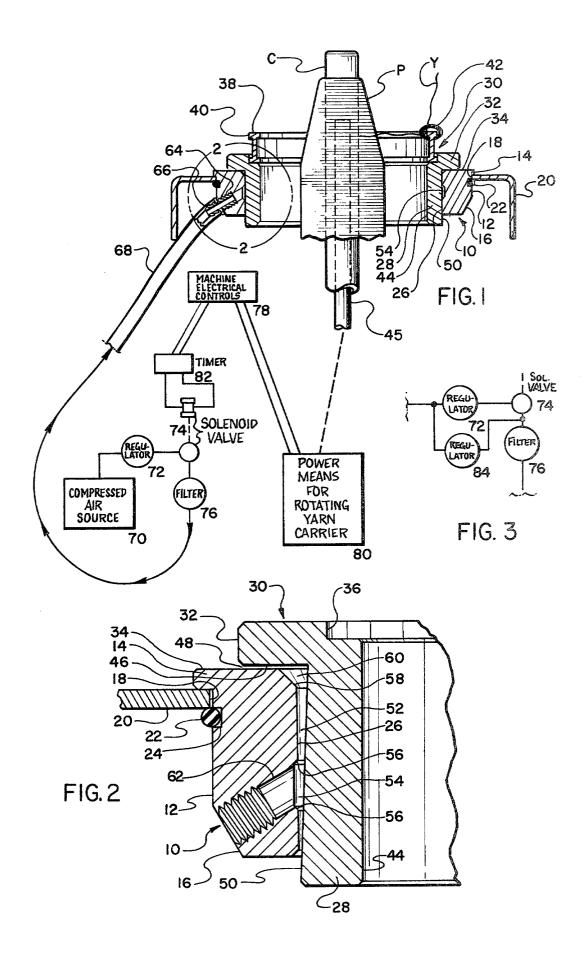
ROTATING RING YARN SPINNING OR TWISTING APPARATUS AND METHOD
