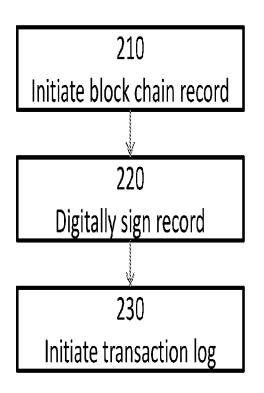
An initiator of a block chain log creates the log by recording the quantities, serial numbers, and description of the smallest saleable unit in a shipment.
