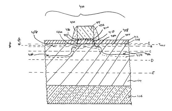
(57) Abstract: Misfit dislocations are selectively placed in layers formed over substrates. Thicknesses of layers may be used to define distances between misfit dislocations and surfaces of layers formed over substrates, as well as placement of misfit dislocations and dislocation arrays with respect to devices subsequently formed on the layers.
